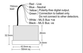
Please Note: The MLS Bus is polarity-conscious unless specified otherwise on the detector/control module.
