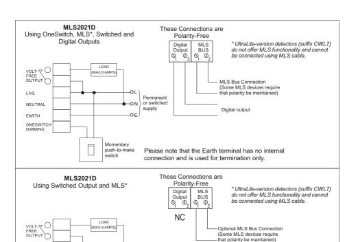
Please note that the Earth terminal has no internal connection and is used for termination only.
