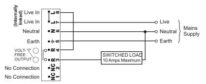
**Note:** A means of disconnection must be incorporated into the fixed wiring in accordance with the current wiring regulations.
