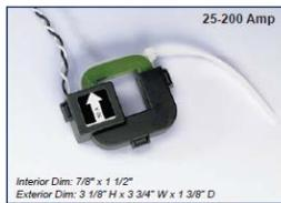
Split core current sensors can be taken apart, or 'split' into halves, which allows the installer leave the power on the circuit during installation. This saves installation time, and for critical loads that cannot be switched off, split core current sensors are essential. Highly accurate the split core current sensors are a little larger than solid core current sensors.
