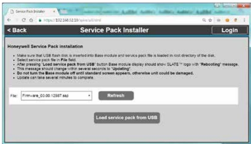
Press „ Load service pack from USB“ button to initiate the installation process. Please note that installation cannot be cancelled once started. Never reboot the unit during installation if not prompted to do so.
