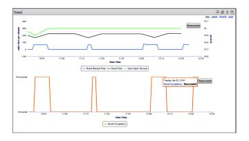
This example of a hood usage trend graph from Phoenix Controls Supervisor dashboard shows hood flow, wasted flow, and sash open percent as well as occupancy of the hood.
