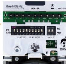
**Snap-Select EOL Resistors:** Auto-calibrates sensor settings, preventing incorrect wiring and reducing installation times.
