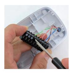
**Easy connection:**The plug-in connector can even be removed from the socket to facilitate the cabling.
