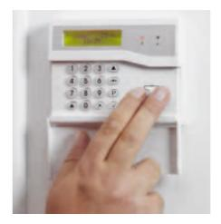
Explain to the customer about the panic alarm. By pressing the two buttons indicated will initiate the internal and external sounders.
