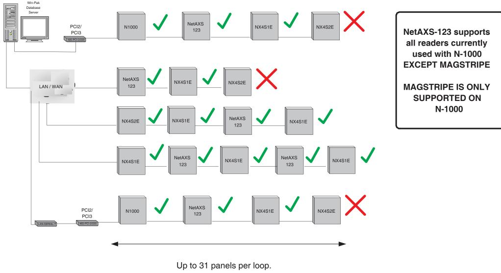
Up to 1500m when using Belden 9842 or equivalent.
