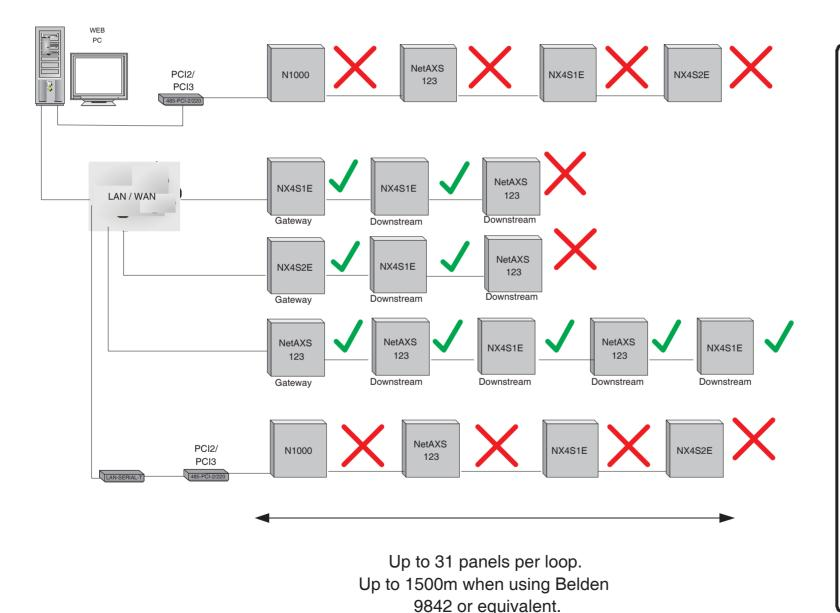
The first panel on any one given loop is called the Gateway. All other panels on that loop are called Downstream panels.
