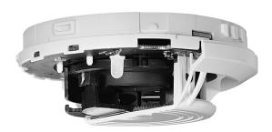
Unique Omni Sensor design features a mechanically integrated photoelectronic and ionization shared volume smoke chamber
