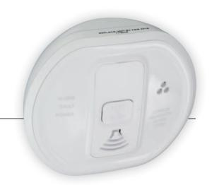
The CO8M is a Carbon Monoxide (CO) alarm device. The front panel is fitted with lights to indicate alarm, operation, fault, test and diagnostic conditions. The CO8M uses a proven electrochemical sensor which has been individually calibrated and tested in Carbon Monoxide (CO) gas to ensure accuracy. When dangerous levels of Carbon Monoxide are detected, the siren will sound and the red alarm light will flash to indicate an alarm status.
