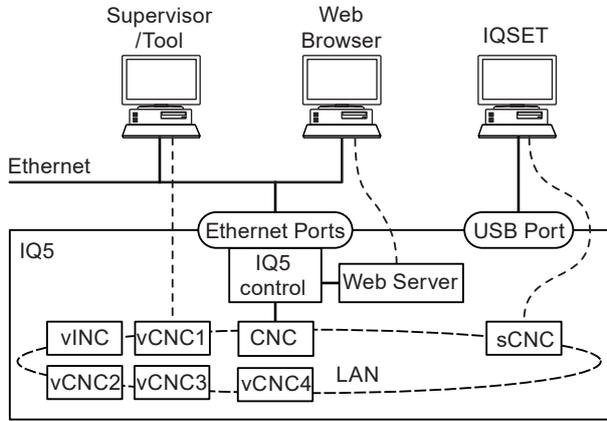
**Default CNC Addressing:** The IQ5 device (outstation) address is factory-set (in the Address module) as follows:
