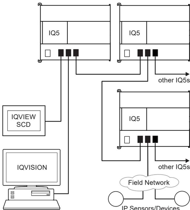
Using one of the ports the IQ5 can form a Trend LAN with other IQ5-compatible devices over an Ethernet network:
