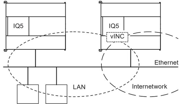
In addition, the IQ5 has the ability to join an internetwork using its virtual internetwork node controller (vINC).
