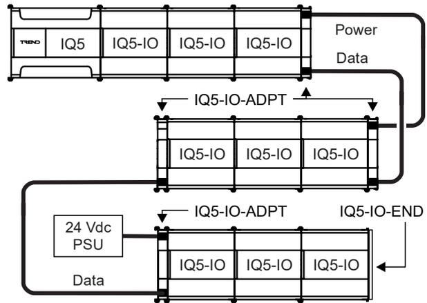
A protective cover (IQ5-IO-END) is supplied with the IQ5 to protect the T1L contacts when not in use. This can be removed and fitted to cover the contacts of the last module on the T1L bus. Spare covers are also available.
