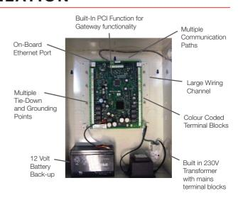
Eliminate additional set-up costs with intuitive installation – one panel does it all.
