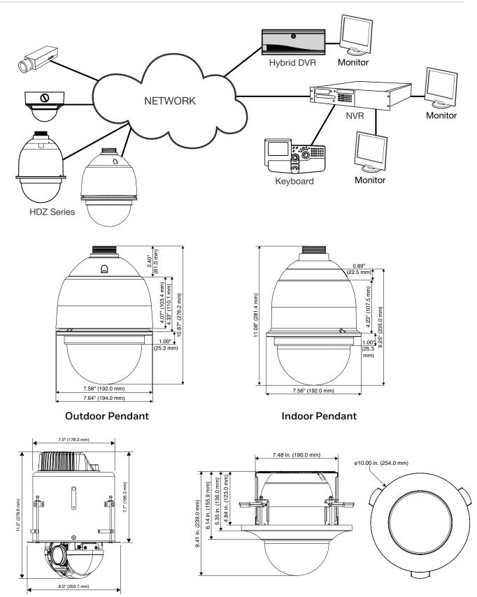
Using In-Ceiling Back Can Housing (HDZHINKIT)
