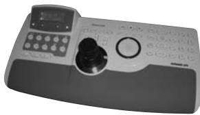
Connectivity to the NetCPU is either through RS422 or Ethernet.
