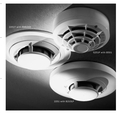
System Sensor 200 Series intelligent plug-in smoke detectors with integral communication provide features that surpass conventional detectors. Detector sensitivity can be programmed in the control panel software. Sensitivity is continuously monitored and reported to the panel. Point ID capability allows each detector's address to be set with decade address switches, providing exact detector locations for selective maintenance when chamber contamination reaches an unacceptable level.
