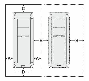
Fig. 4. Distances to ensure proper cooling
