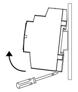
Dismount unit by levering the lower catch open with a screwdriver, pulling the lower edge forward, and unhooking from the top of the DIN rail.
