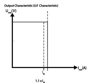
Current overload protection is constant current at (1.1 x nominal current).
