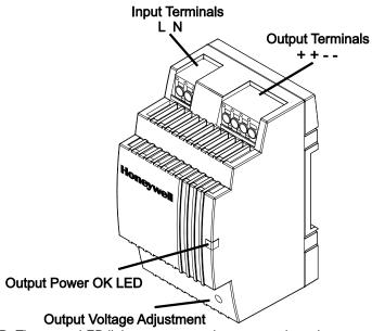
Output Power OK LED: The green LED lights as soon as the output voltage is present.
