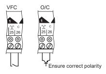
The volt free contact has a nominal wetting current of 270  $\mu$ A. The input is ON when the contact is closed. There is no polarity.
