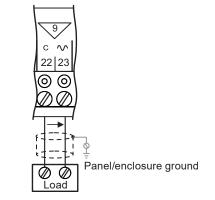
Use 2-wire twisted screened cable for wiring the outputs, with the screen connected to the panel/enclosure ground and unterminated at far end. Connect the return to the C terminal (e.g. 22 C) not to an input common.
