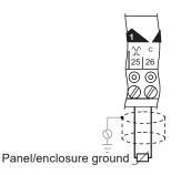
Voltage input: Used with a 0 to 10 Vdc source.
