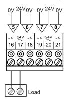
**/230:** All /230 controllers except IQECO32 have four synthesised 24 Vac outputs. Terminals and example wiring.
