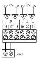
The electrical characteristic of the synthesised 24Vac output is approximately as shown below. Loads should be assessed against this before they are used with /230 controllers.
