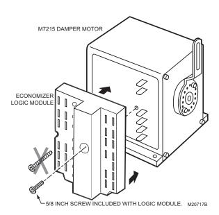
Fig. 2. Direct mounting of module.
