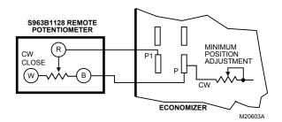
Fig. 6. S963B1128 Remote Potentiometer used with logic module for remote damper control.
