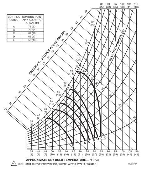
Fig. 8. W7212C performance characteristics for enthalpy changeover settings
