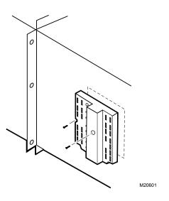
Fig. 3. Mounting the module on sheet metal.
