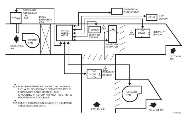
Fig. 4. Representative locations of connected economizer system devices.
