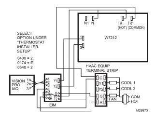
Fig. 17. Vision Pro IAQ with EIM connected to a W7212 Economizer (With Morning Warm-up Enabled)
