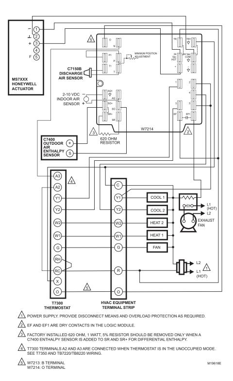
Fig. 15. W7213, W7214 controlling heat pump system.
