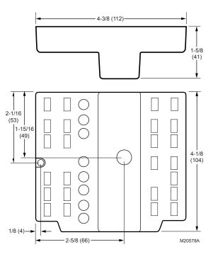
Fig. 1. Logic module dimensions in in. (mm).
