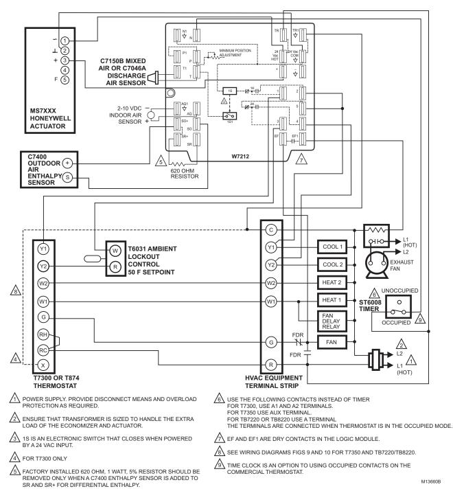
Fig. 13. W7212 used in two-stage cooling system with Honeywell Series 72 Actuator and time clock for occupancy.
