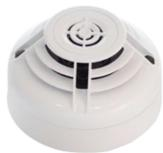
The sensing elements of all three heat sensors are panel controllable through the Advanced Protocol so the sensitivity thresholds of each element can be changed by the panel offering the ability to customise the device for the changing use of the area it is protecting. The detectors have two integral tri-colour LEDs that provide 360° local visual indication of the device status. The LEDs are programmable with static or blinking red, amber and green status indications available.
