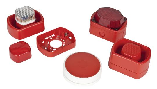
Notifier audible and visual warning devices offer a coordinated range of products to meet the requirements of fire alarm systems. The sounder range has been designed to meet EN54 Pt.3 and features four and fourteen tone models in both standard and detector base formats. Strobes use high performance xenon tubes to produce an intense flash of light, with low current draw. Xenon strobe units are available as separate units or combined with sounders.
