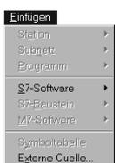
Import takes place with the function "Insert, External Source" from STEP 7 programming software. When "Process, Translate" is then selected, the relevant data blocks containing the stored HTML pages and pictures are integrated by STEP 7 programming software into the user program.
