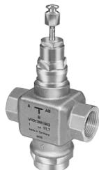
The V5013N is a three-way threaded globe valve for control of hot water, cold water, and glycol solutions (up to 50 percent concentration) in heating or cooling HVAC applications. The valve is used for mixing service to direct flow from one of two inlets to a common outlet in two-position or modulating control systems.
