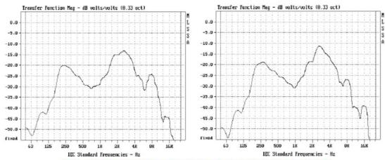
Note: The wide band frequency response is derived using MLS methods
