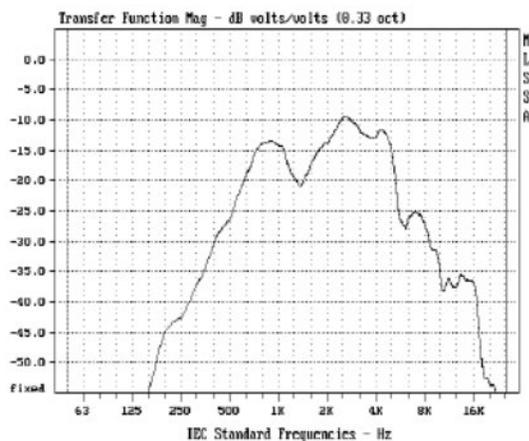
Note: The wide band frequency response is derived using MLS methods
