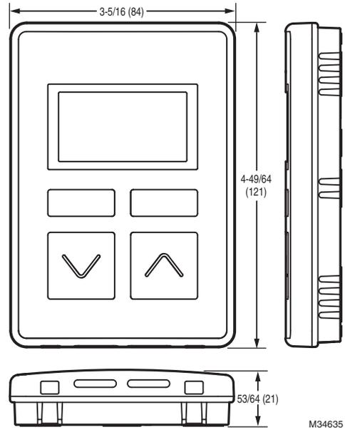
**Fig. 4. LCD Wall Module dimensions in inches (mm).**
