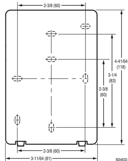
Fig. 2. Subbase mounting holes and locking tabs.
