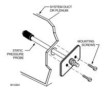
Fig. 2. Mounting static pressure probe.
