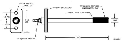
Fig. 1. 32003169-001 Static Pressure Probe dimensions in in. (mm).
