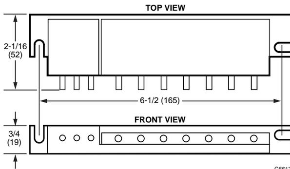
Fig. 1. Dimensions of RP913A.
