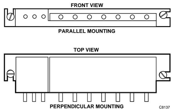
Fig. 3. Parallel and Perpendicular Mounting.
