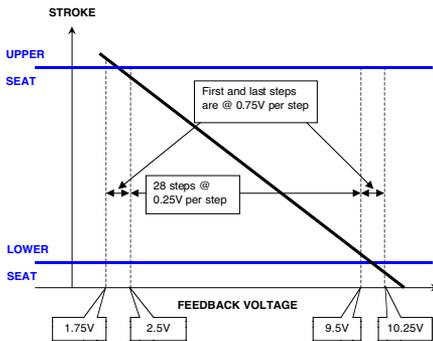
Fig. 4 - Feedback voltage response for reverse acting ML7984
