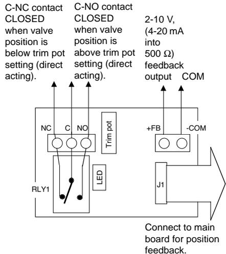
Fig. 2 - Wiring and operation of auxiliary board 272630D
