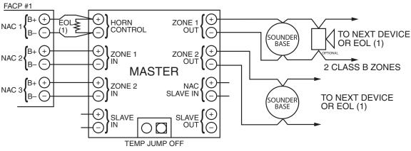
NOTE: Wiring shown for System Sensor MDL Series Sync Module. For additional wiring configurations, see your sync module manual.
