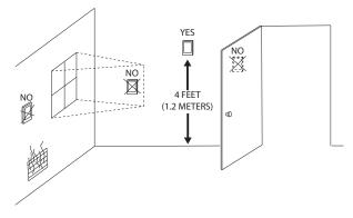
Fig. 1. Typical mounting location of thermostat
