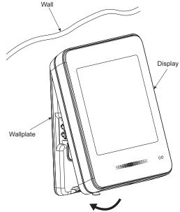
3. Gently tighten the Security screw using a screwdriver by turning it in the clockwise direction (screw torque 0.1Nm).
