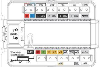
Fig. 6. Thermostat terminal assignments
