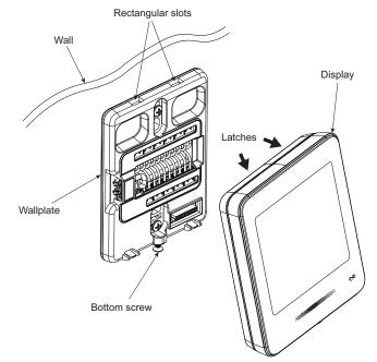
2. Insert the latches onto the wallplate rectangular slots and rotate the display and push it onto wallplate.
