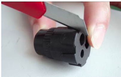
Figure 4 Prepare Compression Gland to Receive Cable
