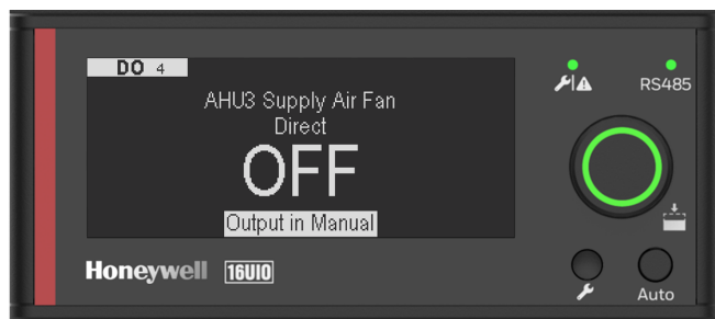
Fig. 17. Channel Screen in Manual Mode
