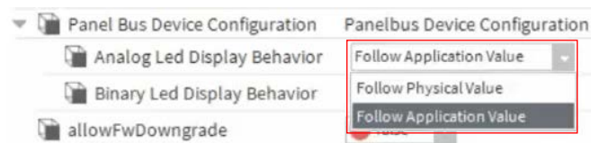
Figure 77. PanelbusNetwork Property Sheet
