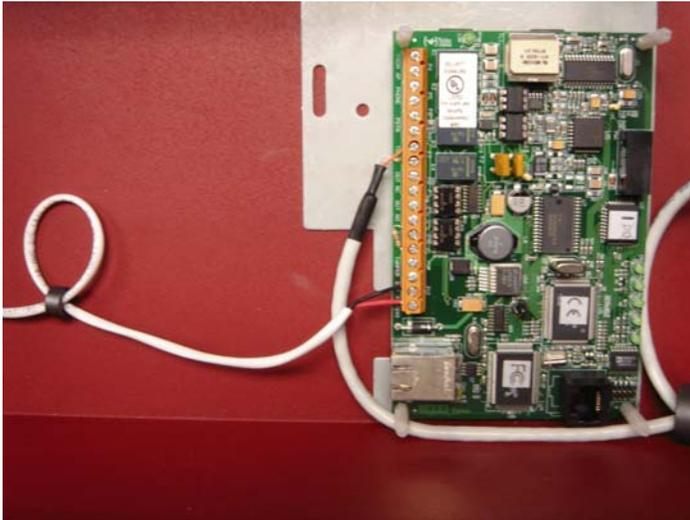
3. Connect 24 VDC from the non-resettable power output of the control panel to the IPDACT terminals marked "GND" and "+12/24VDC". Be careful to observe correct polarity! Run the two conductor power supply wire through the small ferrite ring supplied with the IPDACT.
