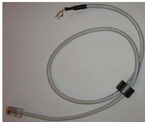
4. Loop the 8 PIN cable supplied with the IPDACT once through the large Ferrite Ring. Note that this cable is NOT used as an Ethernet Cable but to interconnect the dialer output of the panel to the input of the IPDACT. Plug the 8 PIN cable supplied with the IPDACT into the Primary DACT port of the control panel. Connect the other end of this cable to the IPDACT on terminals marked "TO AP."
