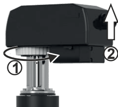
Fig. 5. Dismounting the actuator
