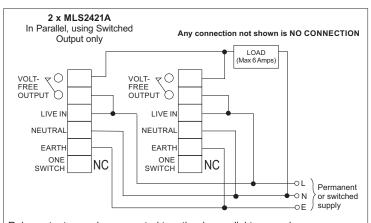
Relay outputs may be connected together in parallel to cover larger areas. however the total load on all combined relay outputs must not exceed 6 Amps.
