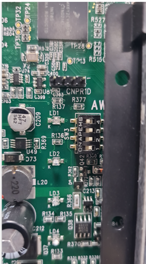
Figure C-79: Switch Position for Firmware Upgrade in AM8200N/8100 Series Panel
