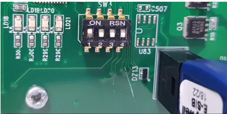
Figure C-70: Switch Position to Retrieve Configuration File in AM CL Series Panels
