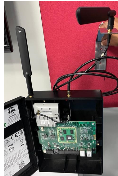
Figure 4-18: Installing Secondary / Diversity Antenna kit
