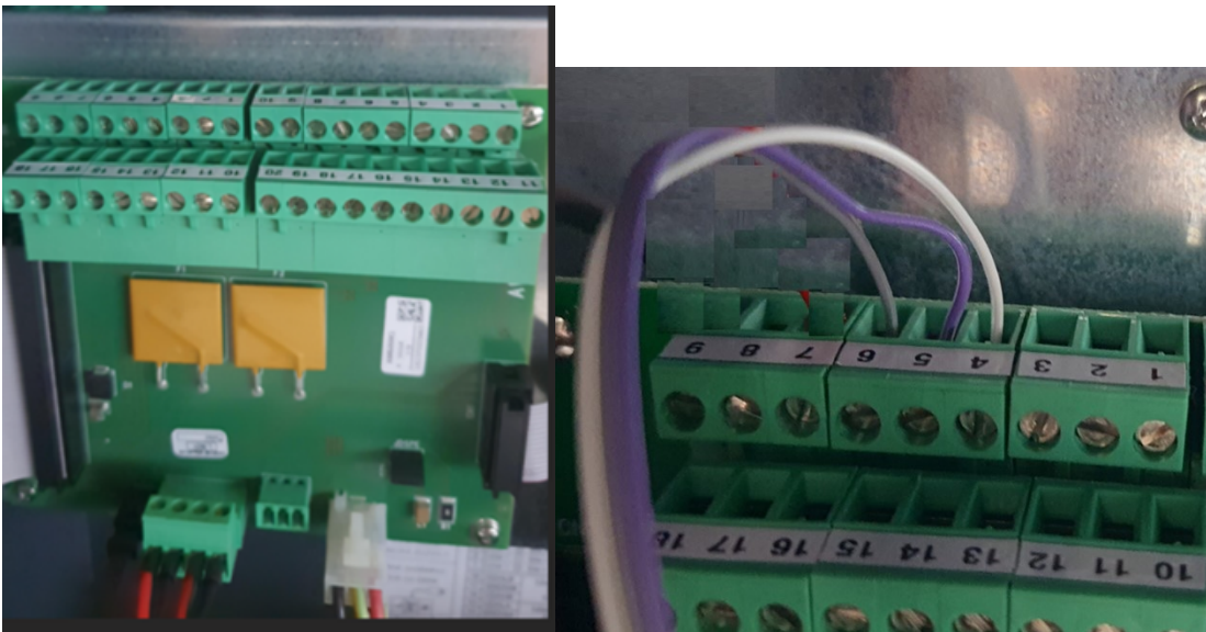
Figure C-62: CNS Connector on AW80US0 Board of Panel with RS-232 Connection AM CL Series Panel
