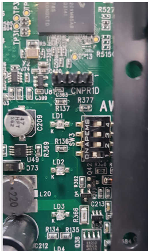
Figure C-71: Switch Position to Retrieve Configuration File in AM8200N/Am8100 Series Panel
