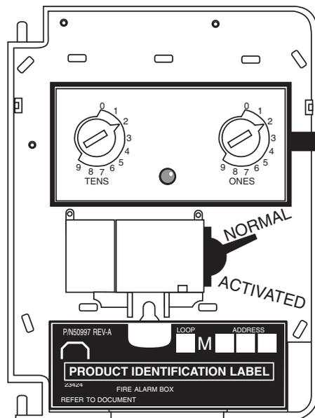
Note - Opening the pull station door will not activate or deactivate the alarm switch.
