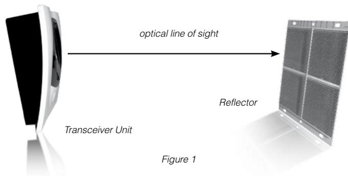
Beam smoke detectors operate on the principle of obscuration. As a smoke field develops, the detector senses the cumulative obscuration – the percentage of light blockage created by a combination of smoke density and the linear distance of the smoke field across the projected light beam. The threshold is typically set by the manufacturer to match the conditions of the installation.
