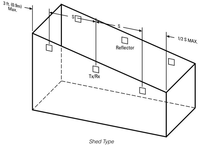
Figures 10 and 11. Mounting on Sloped Ceilings
