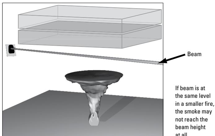
Figures 5, 6, 7. Pre-stratification and detector placement
