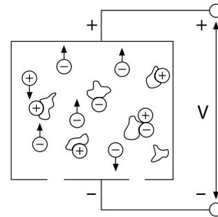
Figure 3: Ion and Particles of Combustion Distribution
