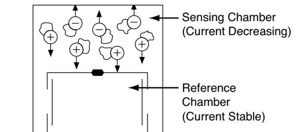
Figure 5: Dual Chamber with Particles of Combustion
