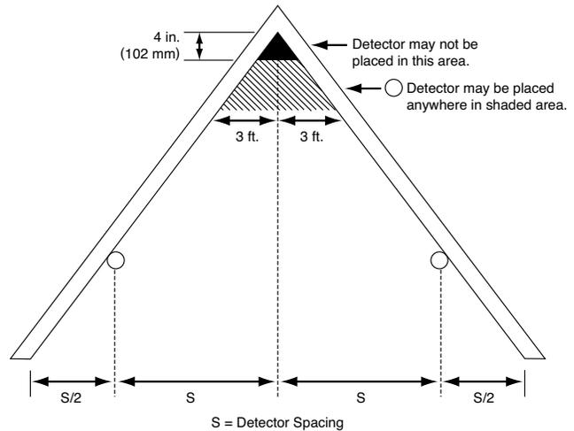
Figure 22: Detector Spacing Layout – Sloped Ceilings (peaked type)
