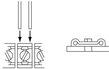
Figure 14: Proper termination
