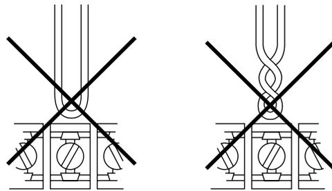
Figure 15: Improper termination
