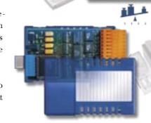
The Saia® PCD weighing module allows precise determining of weight or dosing with very different types of weighing or loading cells that are equipped with a resistance bridge. The signal from the cell is amplified, digitized and filtered in the weighing module, where it is then available to the user as a gross, tare or net weight •
