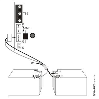
Figure 5 Battery Installation and Connection
