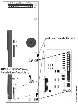
Figure 14 Module Installation - Lower Position
