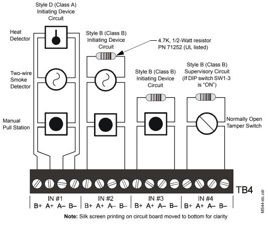
Figure 7 Initiating Device Circuits
