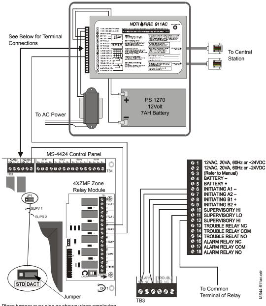
Place jumper over pins as shown when employing a DACT. This directs the control panel to transmit all trouble conditions except AC LOSS.
