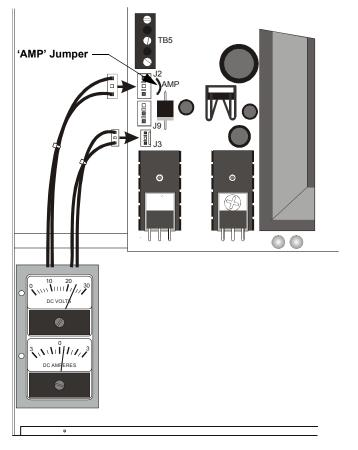
Figure 3 Mounting and Connecting the Meters
