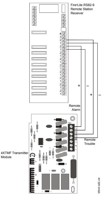
Figure 27 RS82-9 Connections
