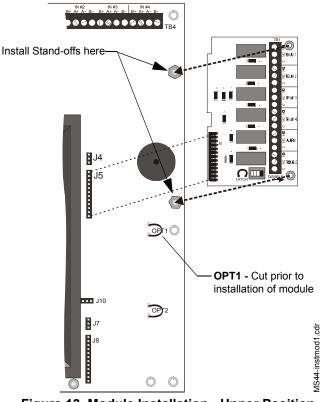
Figure 13 Module Installation - Upper Position
