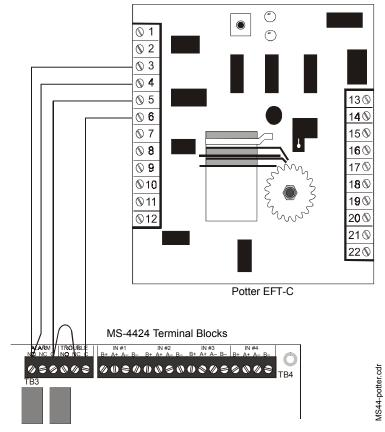
Figure 28 Potter EFT-C Connections
