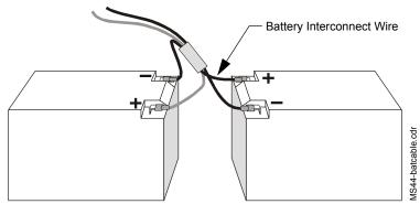
Figure 20 Battery Connections
