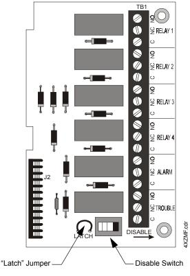
Figure 16 Wiring the Zone Relay Module
