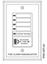
A local trouble sounder and silence switch are also provided. All LED wiring is supervised for open conditions. Any open condition will cause the System Trouble LED to illuminate. Slide-in paper labels permit an easy change of zone information.
