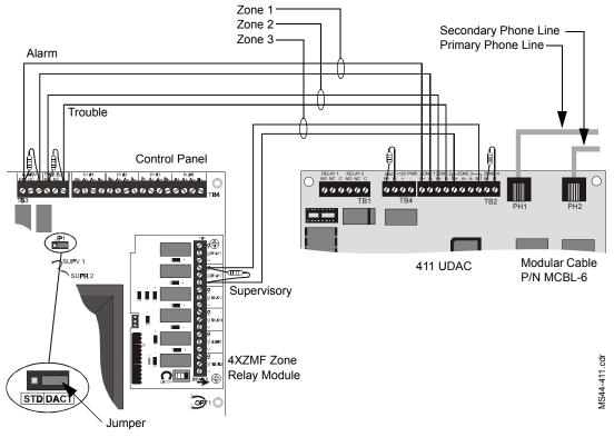
Figure 25 411UDAC Connections
