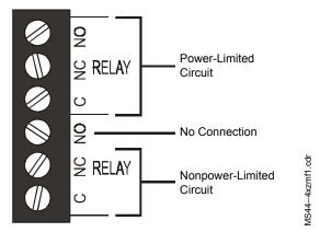
Figure 17 Mixing Power-Limited and Nonpower-Limited Circuits
