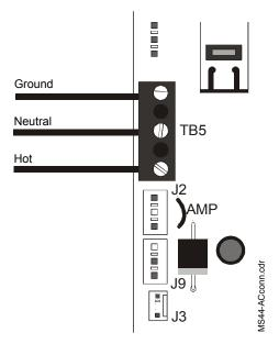
Figure 4 AC Power Connections
