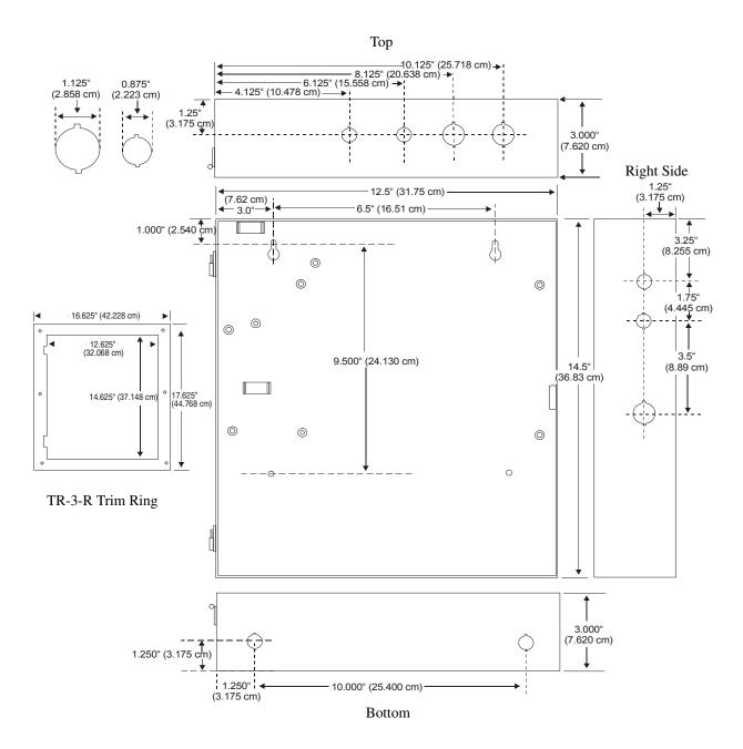
FIGURE 2-2: Backbox and Battery Box
