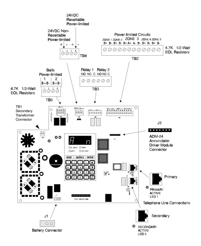
Note: When dressing wires, maintain a minimum of 0.25" distance between conductors to power-limited and nonpower-limited circuits.
