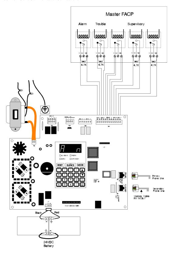
Relays in the master FACP activate various input circuits on the slave communicator. Messages (event codes) programmed for a particular input circuit (channel) will be transmitted to the Central Station upon relay activation.
