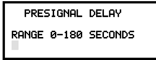
Pre-signal Delay Screen
