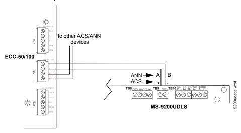
Figure 2.35 FACP Connection to ECC-50/100 Series Audio Panel
