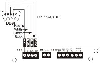
Figure 2.32 Serial Printer and Computer Connections
