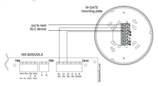
Figure 2.34 W-GATE SLC Connection
