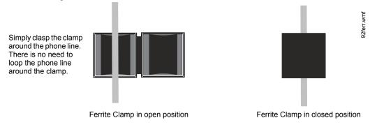
Figure 2.14 Ferrite Clamp Installation
