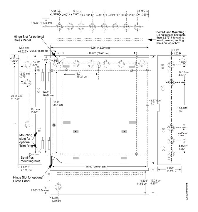
Figure 2.3 MS-9200UDLS Cabinet Mounting
