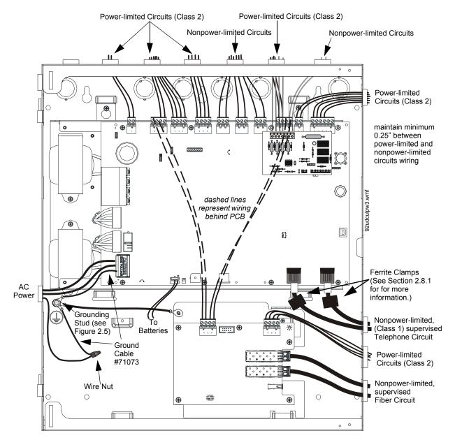
Figure 2.11 Typical UL Power-limited Wiring Requirements
