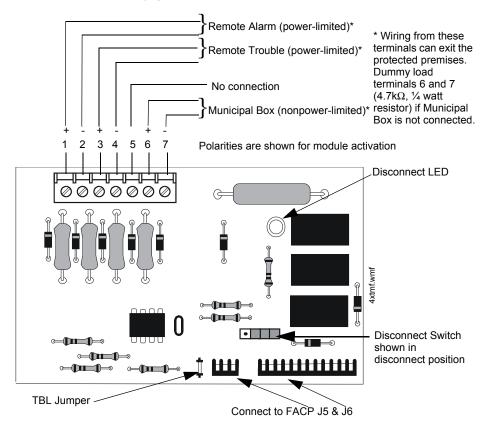
Figure 2.15 4XTMF Transmitter Module
