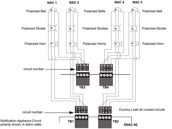
Figure 2.9 NAC Style Z (Class A) Wiring
