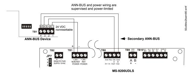
Figure 2.18 Secondary ANN-BUS wiring to ANN-BUS Device
