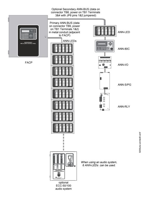
Figure I.2 FACP Maximum Configuration - Eight ANN-LEDs
