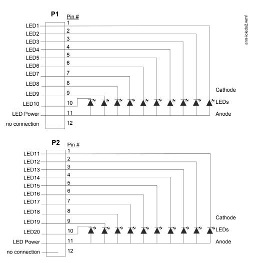
Figure 2.24 ANN-I/O LED Wiring
