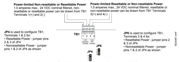
Figure 2.6 Special Application Power Outputs - 24 VDC
