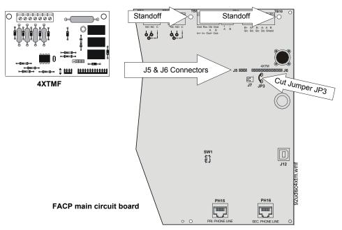
Figure 2.16 4XTMF Connectors to MS-9200UDLS Connectors
