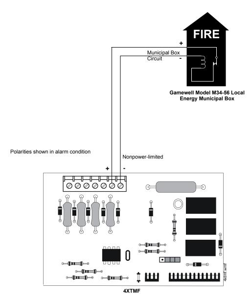
Figure C.1 Municipal Box Connected to 4XTMF Transmitter Module
