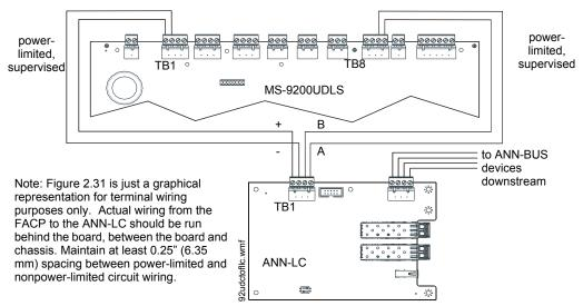
Figure 2.31 Wiring the ANN-LC to the MS-9200UDLS
