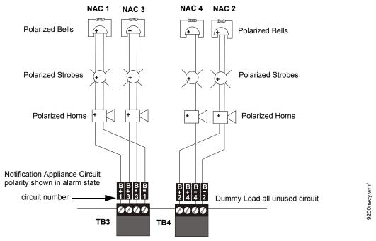
Figure 2.8 NAC Style Y (Class B) Wiring
