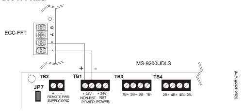
Figure 2.33 ECC-FFT Connections
