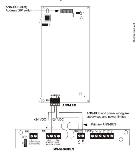
Figure 2.27 ANN-LED Board Layout and Connection to FACP
