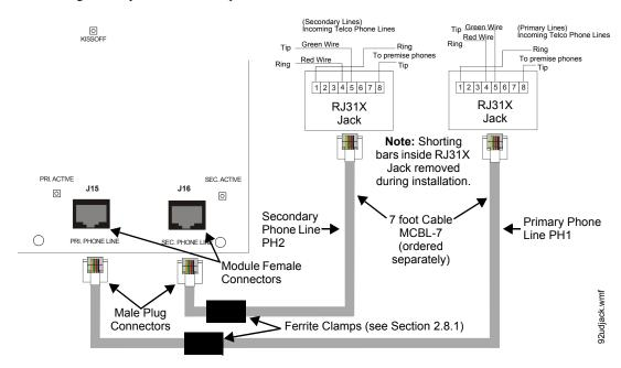
Figure 2.13 Wiring Phone Jacks
