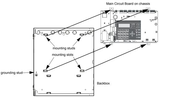
Figure 2.1 MS-9200UDLS Chassis Removal
