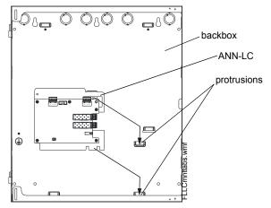
Figure 2.30 Mounting the ANN-LC into the Backbox
