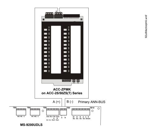
Figure 2.36 FACP Connection to ACC-25/50ZS(T) Series Audio Panel (Legacy)
