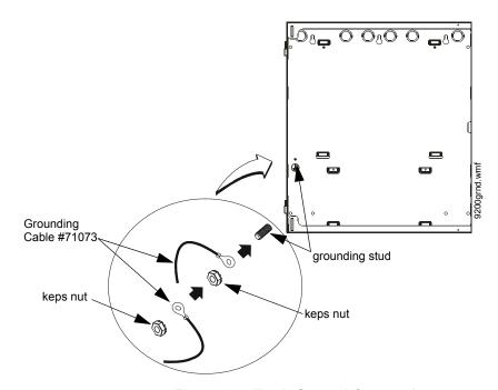
Figure 2.5 Earth Ground Connection
