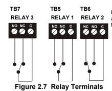
Relay contacts shown <u>with</u> power applied to panel and no active troubles, alarms or supervisories
