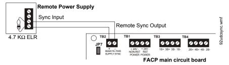
Figure 2.10 Remote Sync Output
