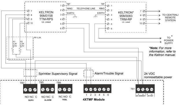
**Note:** Cut TBL jumper on 4XTMF module to send alarm/trouble signal from the same pair or terminals.
