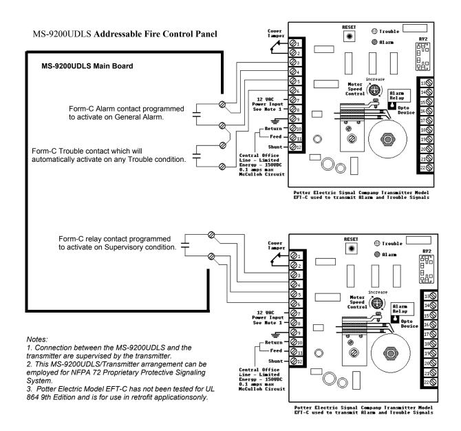
Figure C.3 Proprietary Protective Signaling System
