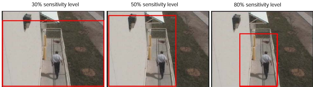
Figure 4 Sensitivity Level Comparison: Normal Field of View
