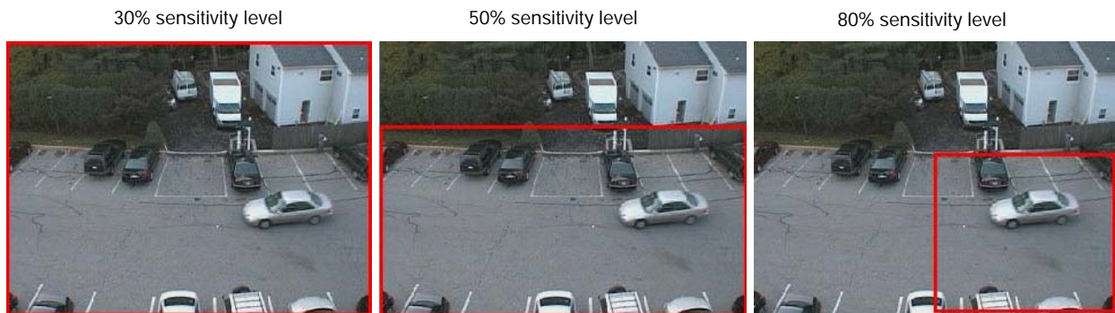
Figure 5 Sensitivity Level Comparison: Wide Field of View
