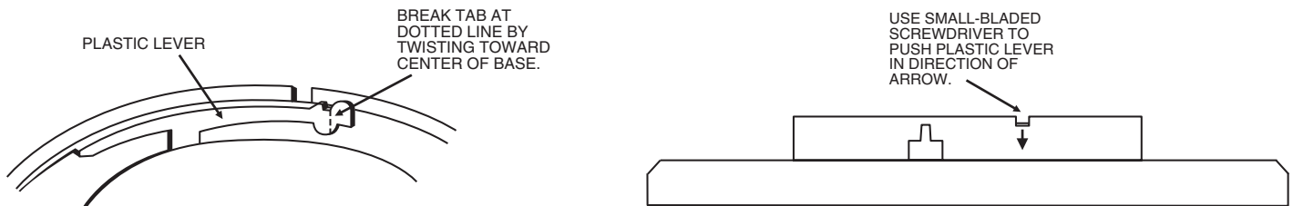
FIGURE 7A. ACTIVATING THE TAMPER-RESIST FEATURE
