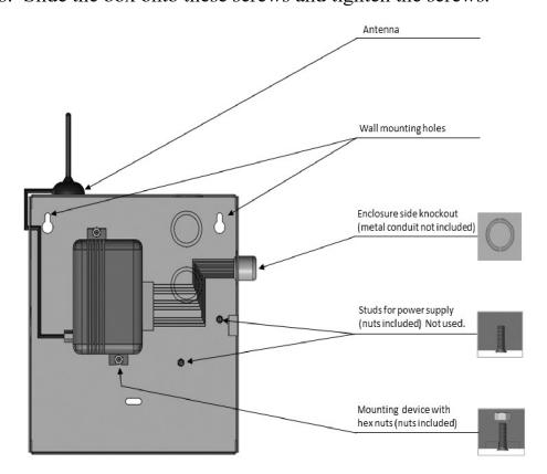
Figure 1: Mounting the Communicator
