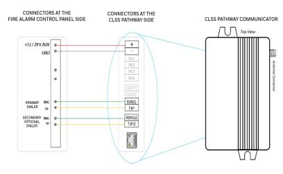
Figure 2: The Wiring Diagram
